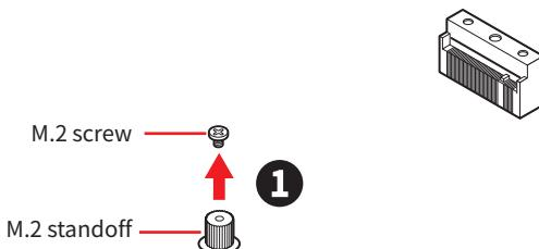
2. Move and fasten the M.2 standoff to the 2260/ 22110 hole. Skip this step if you install 2280 SSD.
