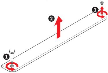
3. If you want to install the 2260/2242 SSD, replace the EZ M.2 Clip II to the 2260/2242 hole. Please note that you have to use the EZ M.2 Chip II Remover to remove and install the EZ M.2 Clip II. If you want to install the 22110 SSD into the M2\_2 slot, please remove the EZ M.2 Clip II in the 2280 hole by EZ M.2 Chip II Remover. Skip this step if you install 2280 SSD.
