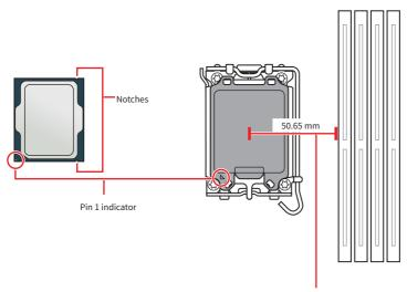
Distance from the center of the CPU socket to the nearest DIMM slot.
