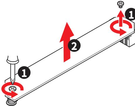
3. If you want to install 22110 M.2 SSD, please remove the EZ M.2 Clip kit in the 2280 screw hole. Skip this step, if you install 2280 SSD.
