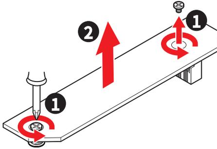
3. If you want to install 2260 M.2 SSD, please install the supplied EZ M.2 Clip kit in the 2260 screw hole. Skip this step, if you install 2280 SSD.
