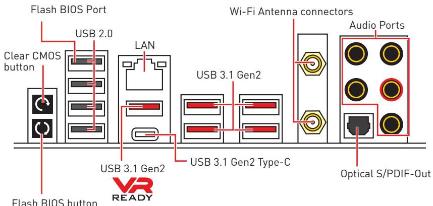
• **Clear CMOS button** - Power off your computer. Press and hold the Clear CMOS button for about 5-10 seconds to reset BIOS to default values.
