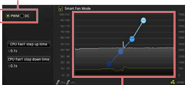
There are gradient points of the fan speed that allow you to adjust fan speed in relation to CPU temperature.
