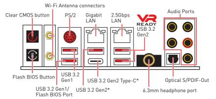
\*USB 3.2 Gen2 (3rd Gen AMD Ryzen™) or USB 3.2 Gen1 (2nd Gen AMD Ryzen™/ Ryzen™ with Radeon™ Vega Graphics and 2nd Gen AMD Ryzen™ with Radeon™ **Graphics**
