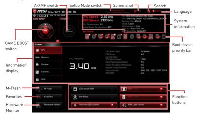
• GAME BOOST switch - click on the center button to switch the GAME BOOST be controlled by software (SW) or hardware (HW) . The inner circle represents the current stage of hardware GAME BOOST and the outer circle stands for software. You can read the abilities of GAME Boost by clicking on the question mark in the right-bottom corner. This function will only be available if the installed processor supports this function.
