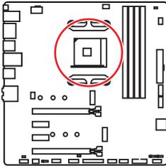
Distance from the center of the CPU to the nearest DIMM slot.
