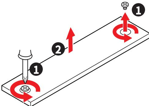
3. If you install 2260 SSD, please use the included **EZ M.2 Clip II Remover** to install the included **EZ M.2 Clip II** in the screw hole. Skip this step if you install 2280 SSD.
