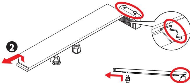
3. If you install 2260 SSD, please use the included **EZ M.2 Clip II Remover** to install the included **EZ M.2 Clip II** in the screw hole. Skip this step if you install 2280 SSD.
