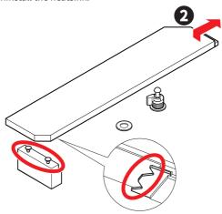
3. If you install 2260 SSD, use the included EZ M.2 Clip II Remover. Place the included EZ M.2 Clip II in the slot, use the remover to screw it in by turning clockwise, and secure it. Skip this step if you install 2280 SSD.
