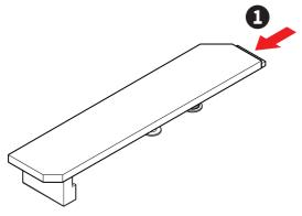
2. Slightly lift up the end part of Screwless M.2 Shield Frozr heatsink and move it forward to uninstall the heatsink.
